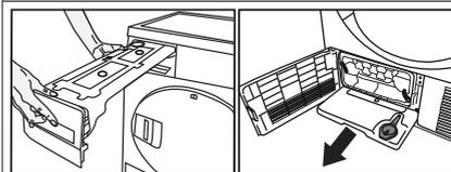
2. Drain the water in the tank.
